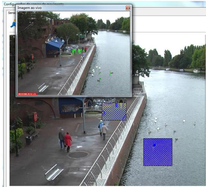
The figure below demonstrates how the motion sensor works with selection of non-motion sensitive areas:
